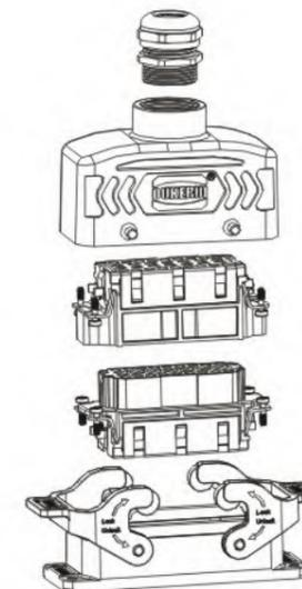
● 开孔安装/Bulkhead mounting
