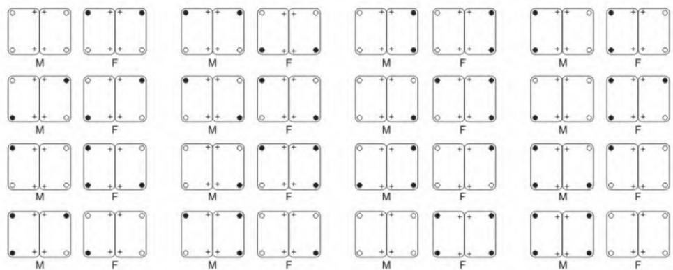
●-导向销/Guide pins    M-公插体/Male connector    ○-导向套/Cuide bush    F-母插体/Female connecto
