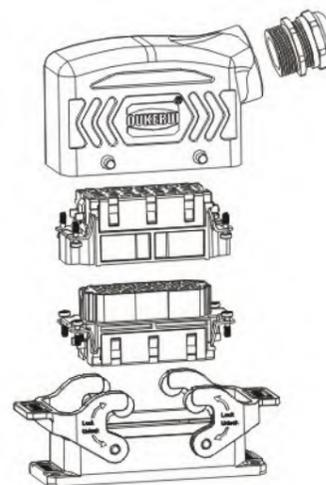
● 开孔安装/Bulkhead mounting
