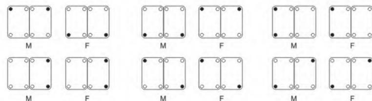
●-编码销/Code pins M-公插体/Male connector ○-正常螺丝/Normal mounting screw F-母插体/Female connecto
